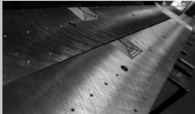
Our standard parallelism is 0.01 mm per meter, and the standard surface finish during fine grinding is Ra = 0.8  $\mu$ m. Micro-precise guide rails are possible depending on the design.
