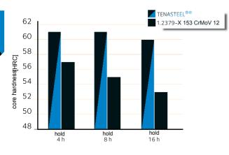
Please note that for nitriding treatment following hardening, it must be tempered at a minimum of 525°C.
