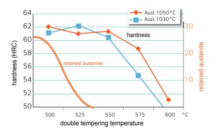
The graph illustrates that a high austenitizing temperature (1,050°C) still results in a hardness of 58 HRC after tempering at 575°C.
